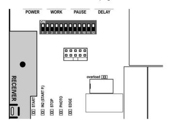
The MR1 receiver module has 4 channels, each with an associated command on the **City7** control unit:
